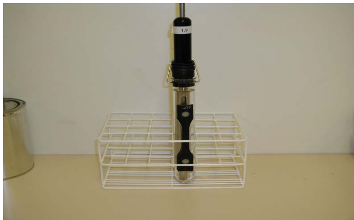
Figure 2 Surface-active solution, Igepal CO-720 at 60 C, stress level 5,0 MPa.
