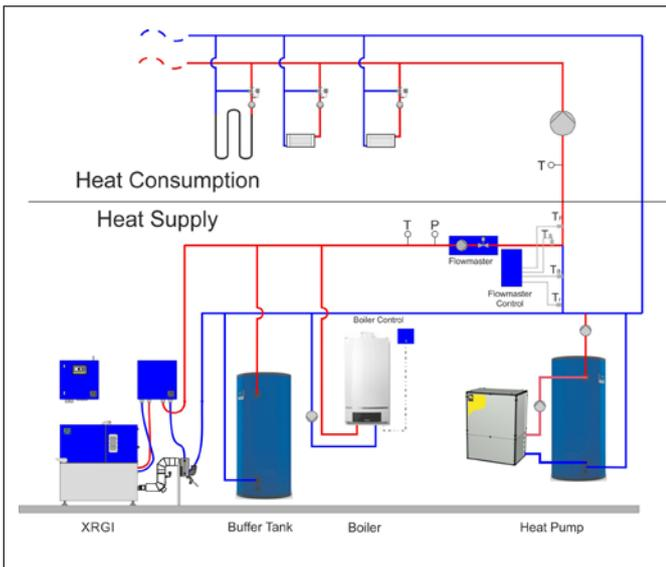
Figure 1. An example of a typical system layout, showing the cogen unit, a heat pump, heat storage units and the necessary controls for creating optimal working conditions for the installation. A peak load boiler is also seen.
