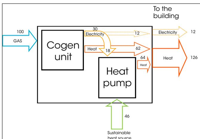
Figure 4. Sankey diagram of the energy flows during operation of both the cogen unit and the heat pump.
