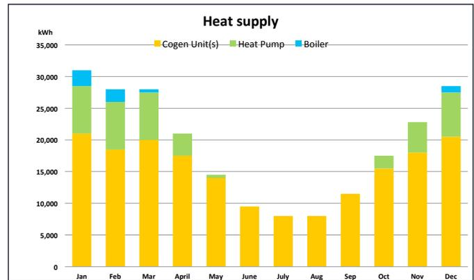
Figure 3. The heat production and the origin of the heat on a monthly basis over a year for a sports centre.
